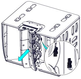
Remove 4 screws to access diaphragm.
