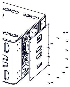
First release the bottom of the HF block, then the top. Be careful not to trap your fingers in the HF guides. Disconnect cable
