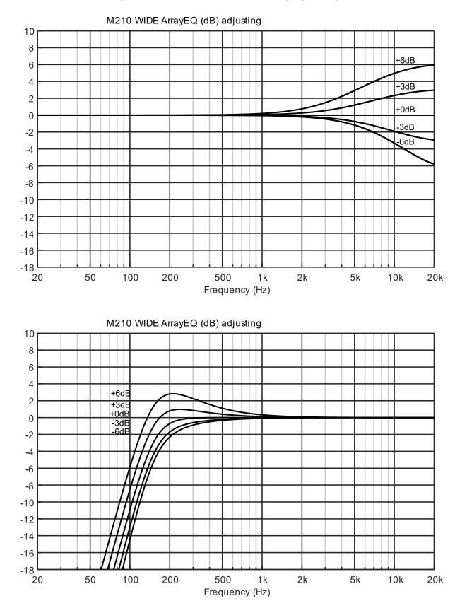
The ArrayEQ allows to adjust the system frequency response in its lower range (see curves below, with different ArrayEq values):
